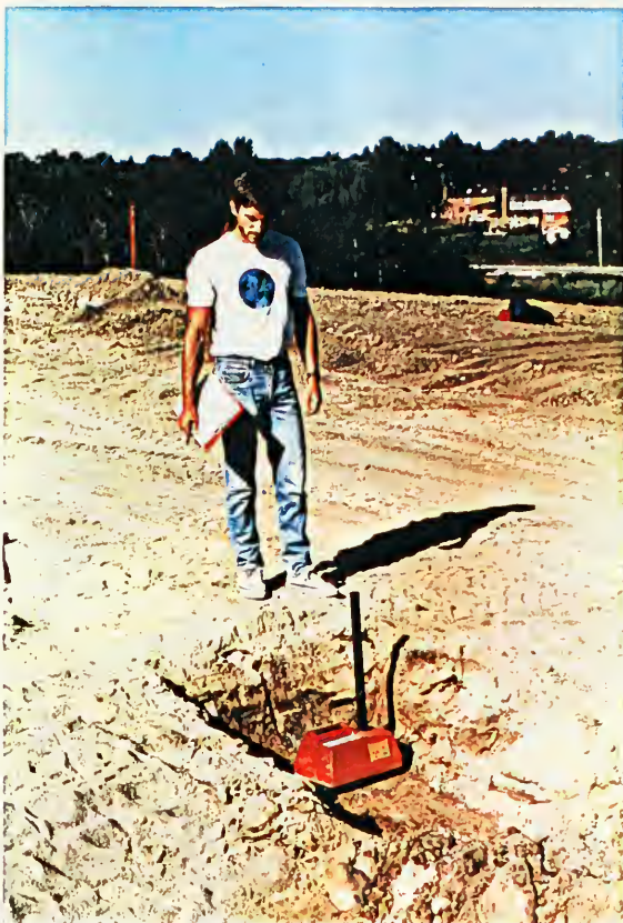
A1: MEASURING EXISTING COVER DENSITY AT 0.3 m (1') INTERVALS
